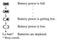
When the batteries are depleted, replace both batteries with new ones.
